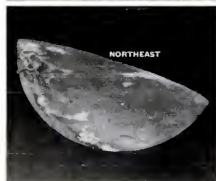
ONE-SECOND SEQUENCE taken as rocket revolved reveals variation in horizon's position which proves missile was tilted in flight. Had rocket been vertical, pictures would have had identical shape.
