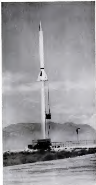
TAKING OFF , the 48-foot rocket rises slowly from launching scaffold, then accelerates to maximum velocity of more than 4,000 mph. The camera began taking pictures as the rocket left the ground and kept on shooting during the entire four and a half minutes that it took the Viking to travel up to 135 miles.
