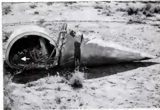
HEAD OF ROCKET was found lying on the desert some 50 miles north of the launching point and a quarter-mile from rest of rocket. Head was deliberately blown off rocket during descent so that it would fall more slowly. The camera (indicated by arrow) was broken, but film was completely undamaged.
